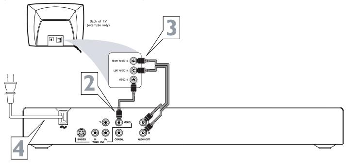
**Disconnect all equipment from the power outlets.** Connect the equipment to the power outlets only after you have finished hooking up everything. Never make or change connections with equipment connected to the power outlet.
